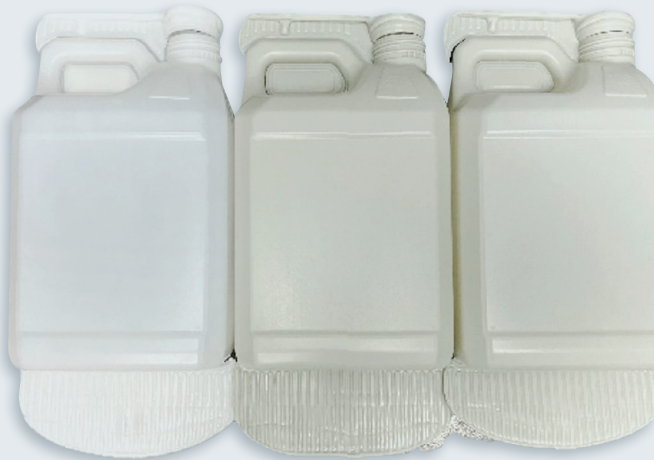
Left: Virgin Bottle, Middle: PCR Bottle, Right: PCR with BAEROPOL T-Blend 1111
