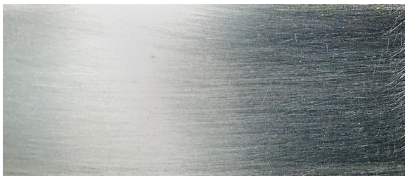
No corrosion as protected by acid scavenger
