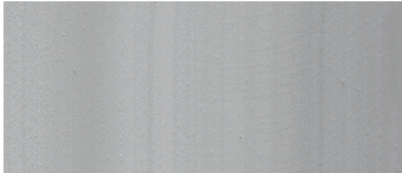
Magnification of PE film surface showing the effect of 1000 ppm of a low FI Calcium stearate from Baerlocher.
